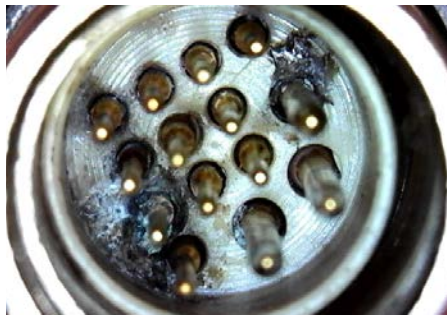
Damaged Contacts from Residual Moisture
