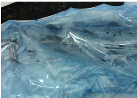
Inadequate Dry Cycle
