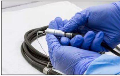
Figure A - Pull back on collar with one hand
