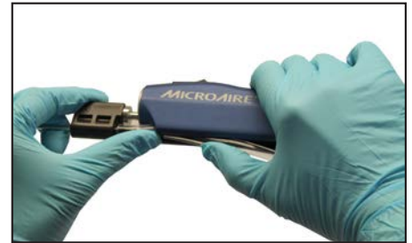
Figure E - Push Tubing into PAL Handpiece
