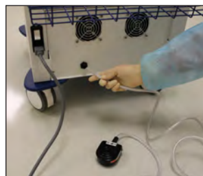
Figure 15 - Connect Foot Pedal to rear of cart to control vacuum pumps
