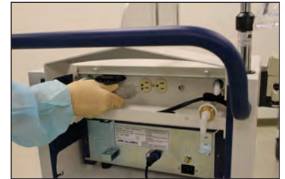
Figure 6 - Plug console into outlet
