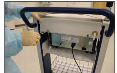
Figure 4 - Unscrew back-cover screws
