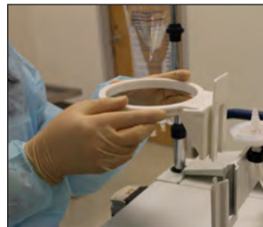
Figure 12 - Install waste canister rings
