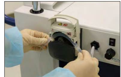
Figure 20 - Insert Infiltration Tubing
