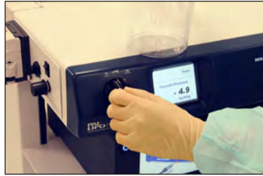
Figure 25 - Three-Way Control Switch
