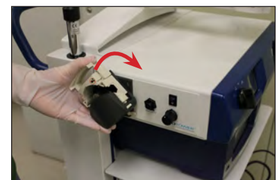
Figure 34 - Rotate the pump head clockwise until it clicks into place.
