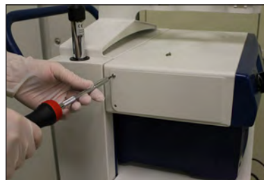
Figure 29 - Remove screws and slide cover towards the back of the cart.
