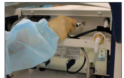
Figure 7 - Attach BNC connector
