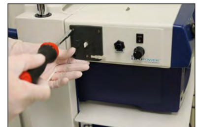
Figure 32 - Replace retaining screws.
