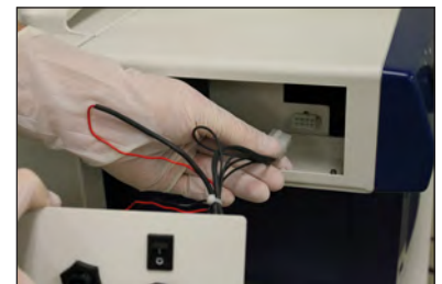
Figure 30 - Connect the electrical harness.
