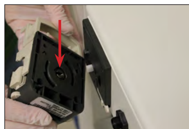
Figure 33 - Align the slot on the pump head with the drive shaft.
