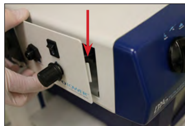
Figure 31 - Insert the Module. Slide it rightward to engage retaining clip.
