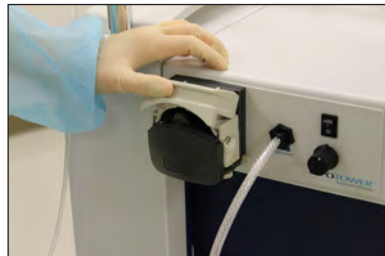
Figure 19 - Open the Tumescient Pump
